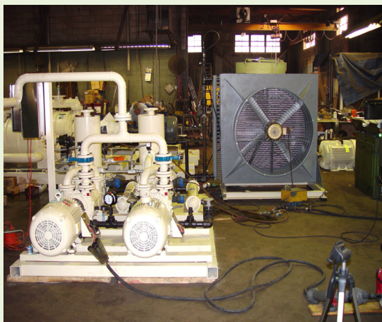
MODEL # 4PSM-240-FR-AC WATERBOX PRIMING SYSTEM (BEING SET-UP FOR RUN TESTING)
